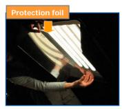
Placing special **infrared protection foil** between the lights and exposed materials. The foil will absorb a considerable part of the generated heat.
