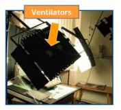
Placing **small ventilators** behind the lights. The air will take the heat out of this space.
